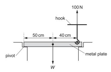
An upward force of 100 N is needed to lift the metal plate about the pivot, as shown.
