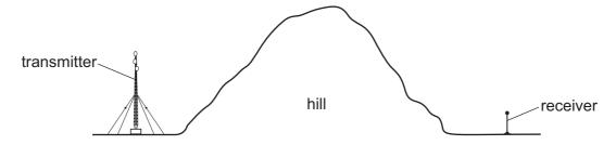
The receiver picks up the signal from the transmitter even though the radio waves do not travel through the hill.
