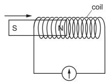
The needle of the galvanometer moves.
